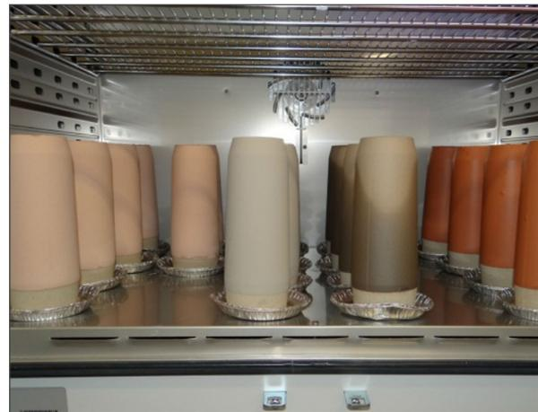
(a) Drying coated cores in an oven
